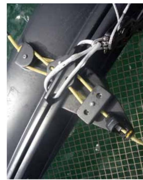
The simple single-line traveller system makes it easy to haul the mainsheet car up the track without friction from the leeward side
