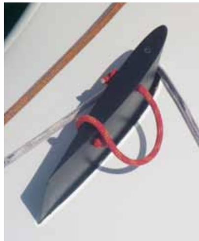
The daggerboards have simple rope handles to raise or lower them, keeping weight down
