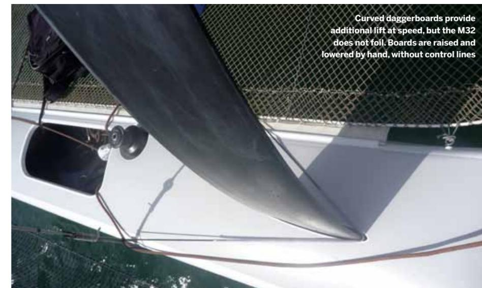
Curved daggerboards provide additional lift at speed, but the M32 does not foil. Boards are raised and lowered by hand, without control lines
