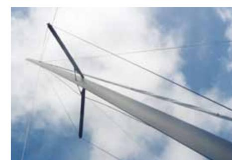
The rotating aerofoil-section carbon mast has one set of spreaders with diamonds that are tensioned by a single nut under the mast
