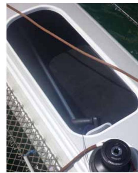
A simple, shallow crew cockpit makes it easy to brace yourself when using the non-self-tailing winch for the Code 0 sheet. There's little else to put on it!
